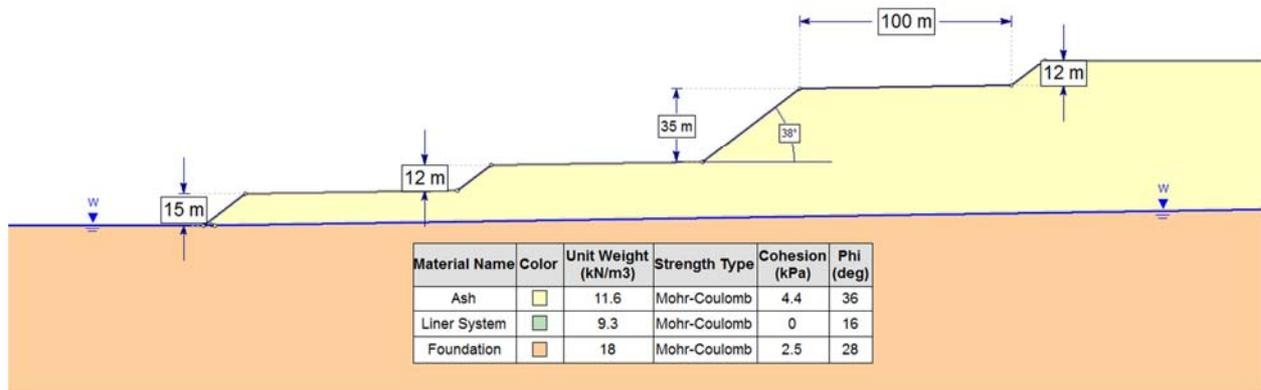
Figure 1: Modelled Site H Ash Dump Configuration
