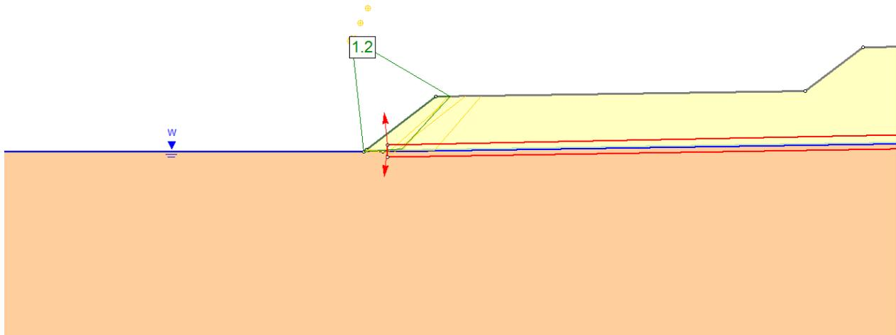
Figure 2: Block-Type Failure at Dump Toe
