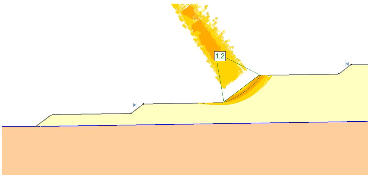
Figure 3: Circular Failure at Mid-Slope Bench
